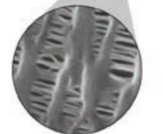
Hydrophobic membrane with pores approx. 0.03 μm
