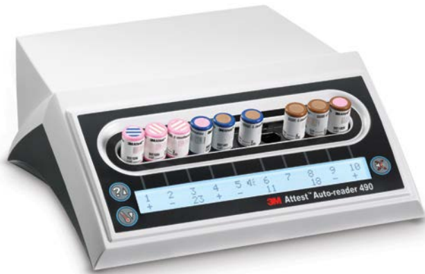
Figure 5. Image of the 3M™ Attest™ Auto-reader 490
