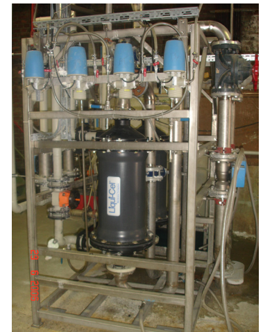
Figure 1. 3M™ Liqui-Cel™ Membrane Contactors treat ammonia wastewater in a European facility
